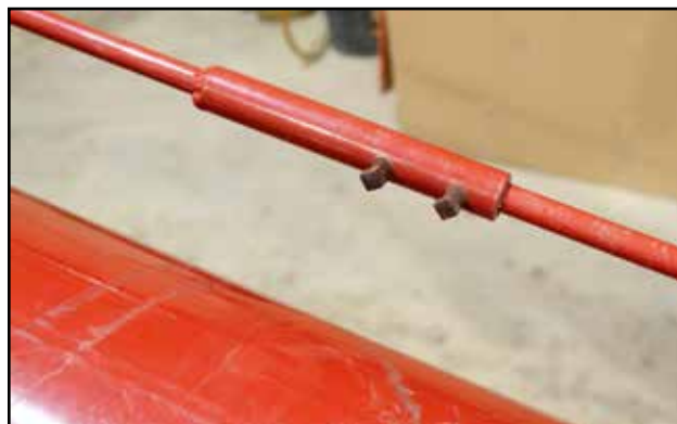
Fig 44 - Set screws to lock rods in place
