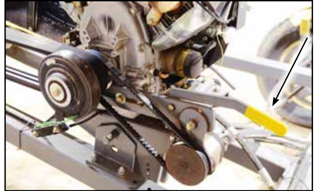
Fig 26 - Pump belt and over-centre cam
