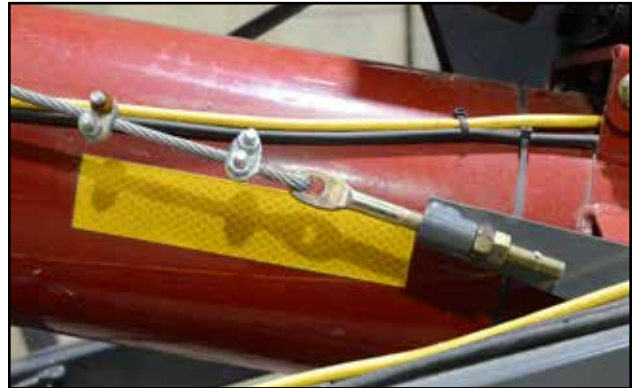
Fig 41 - Adjusting eyebolts at bottom of cable
