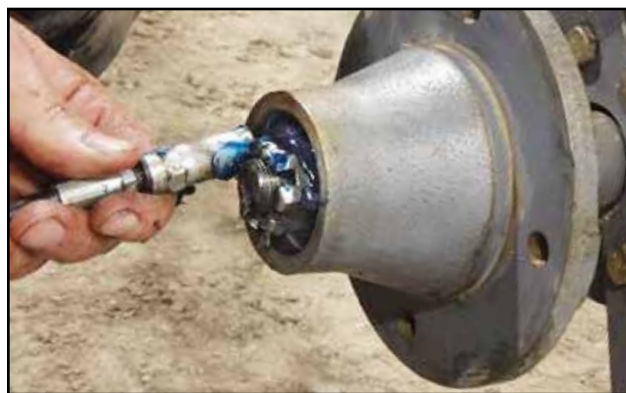
Fig 38 - Fill hub with grease
