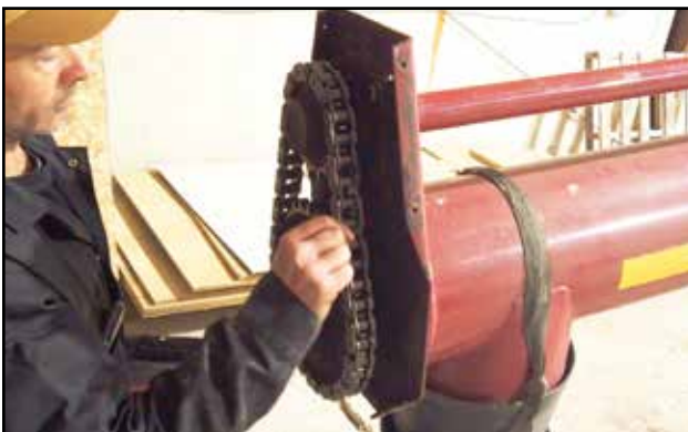
Fig 35 - Inspect chain and sprockets
